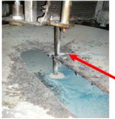
Picture 1 (Rotating shaft in contact with removable lid)
