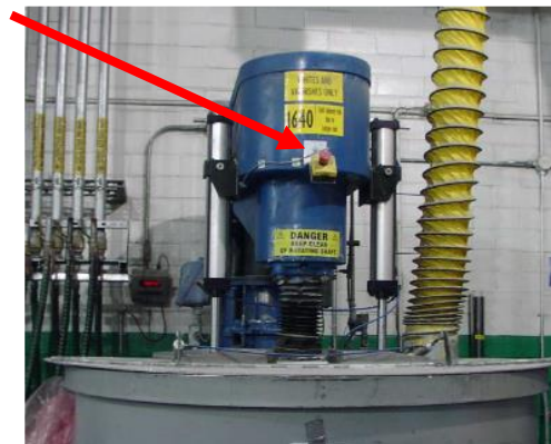
Picture 10 (Example of Emergency Stop for the manual batch operation)
