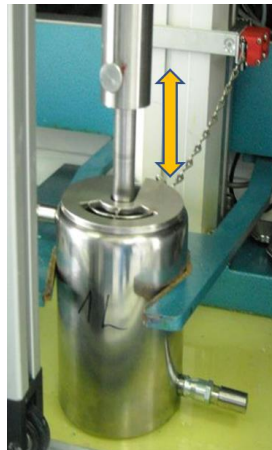
Picture 6 (Shaft protection and cover interlock)
