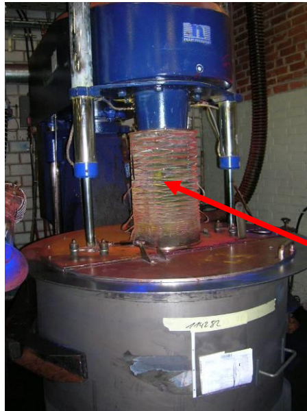
Picture 2 (Permanently installed lid with a sleeve)
